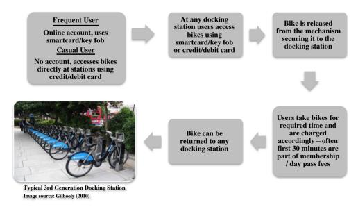
Fig. 1. System diagram - typical third-generation bikesharing system (Gilhooly, 2010).
